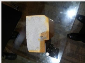
Cut section of frame filled with CLC
